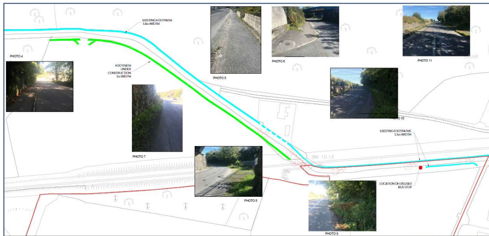
Figure 2-8: Footpath Existing (Blue) and Under Construction (Green) to the North of the Application Site (extract from drawing 10690-2013_Rev B)
